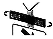
Rotate the light bar towards the incoming vehicle lane, independent of the wire hole location.
